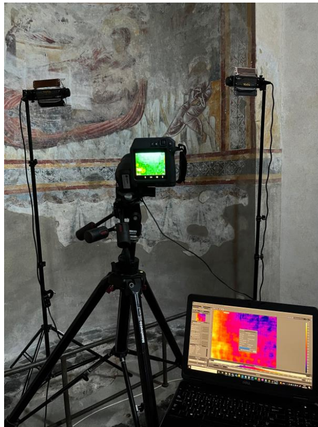
Fig. 2. Measurement rig with thermal imaging camera, halogen lamps and computer
